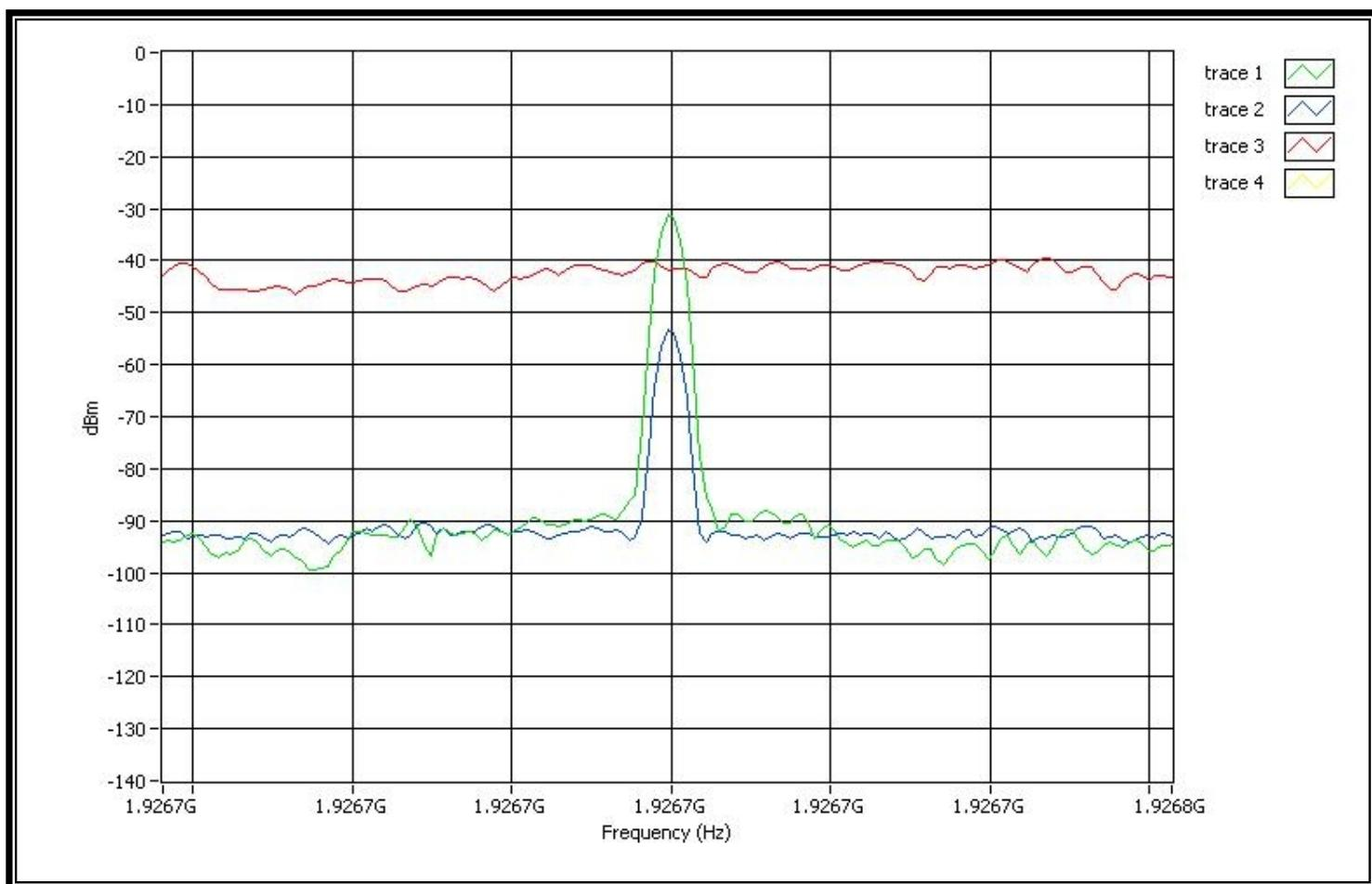
Note1: Trace1 (green) is the interference on all 5 carriers. The level is  $T_u+U_m+10$ dB.
