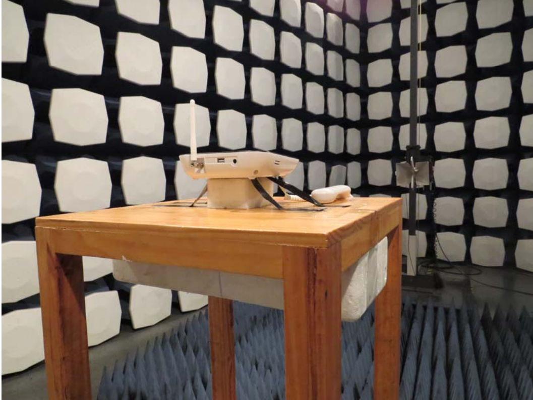
Picture 2: Radiated Spurious Emissions Test setup
