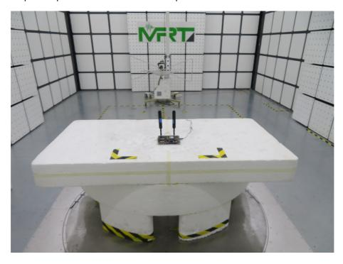
Description: Spurious Emissions Test Setup for above 1GHz
