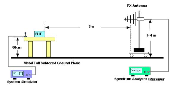
For radiated test above 1GHz
