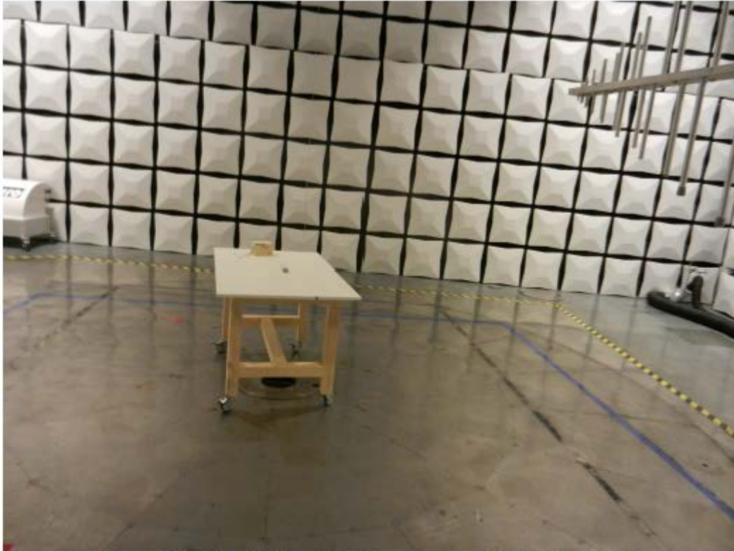
Figure 78 – Test Setup for frequencies 30 MHz – 1 GHz
