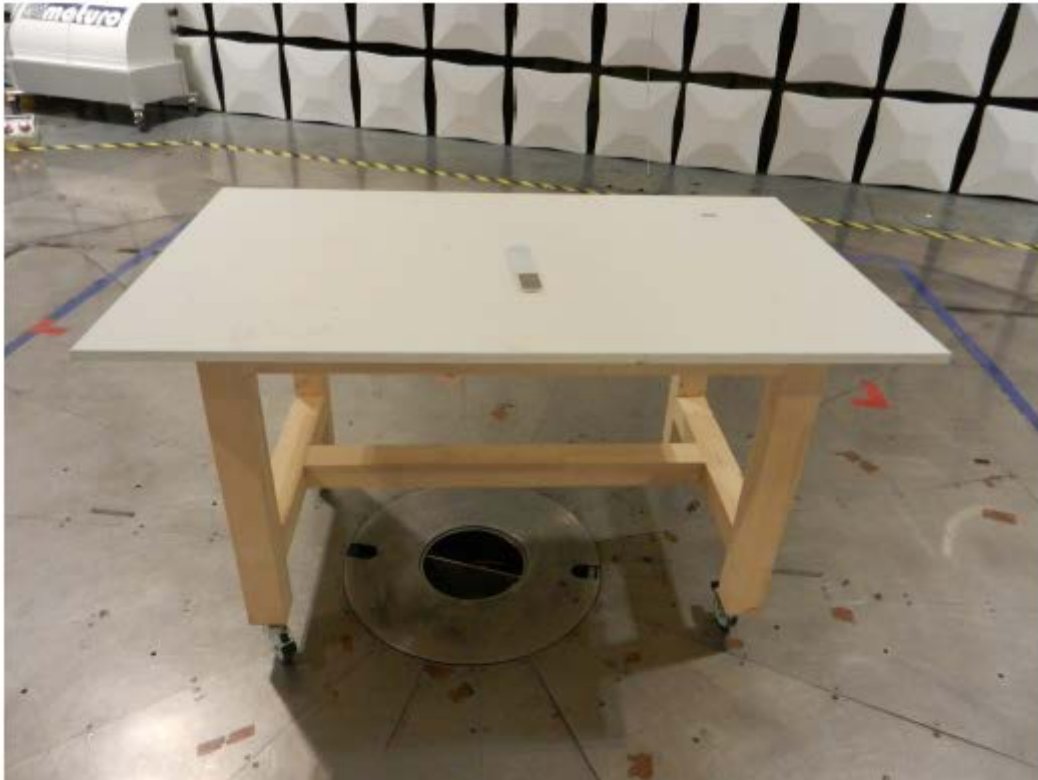
Figure 72 – Test Setup for frequencies 9 kHz – 30 MHz
