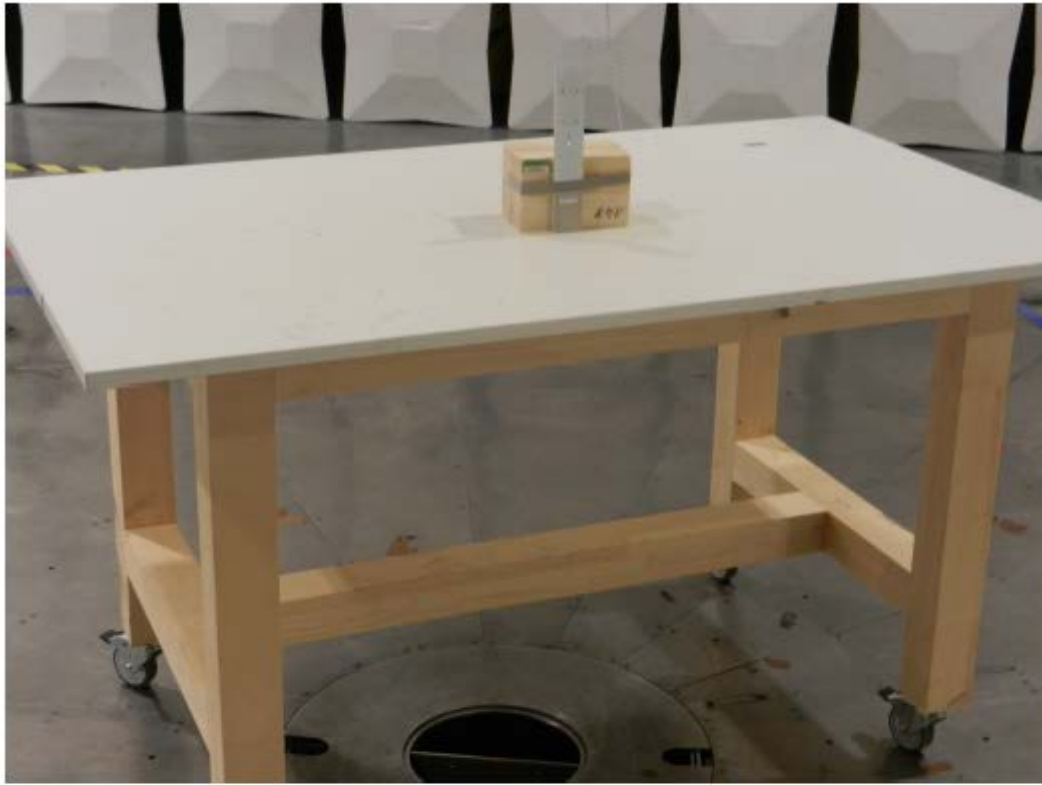
Figure 76 – Test Setup for frequencies 9 kHz – 30 MHz
