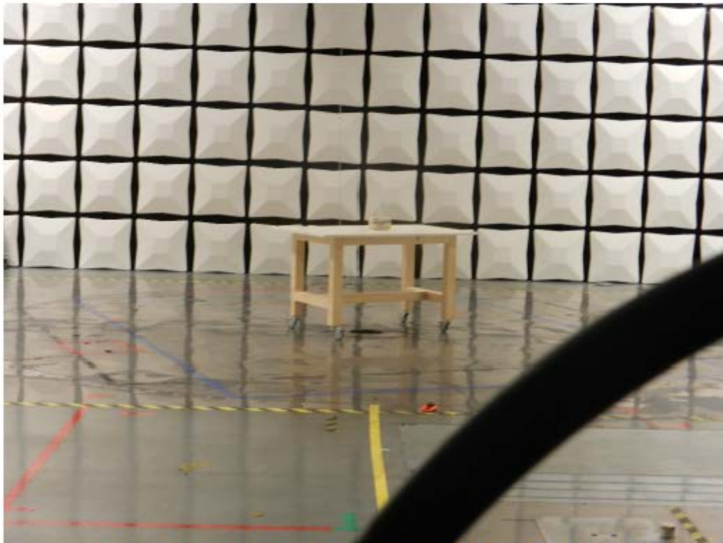
Figure 77 – Test Setup for frequencies 9 kHz – 30 MHz
