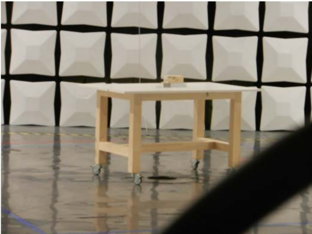
Figure 75 – Test Setup for frequencies 9 kHz – 30 MHz
