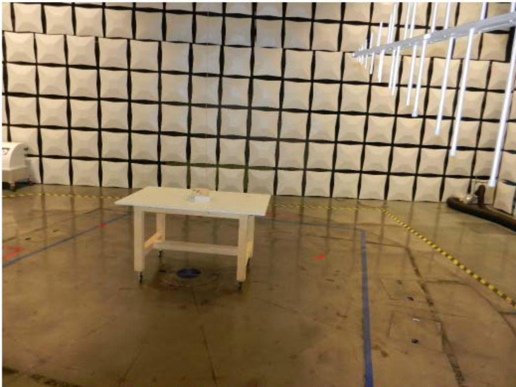
Figure 79 – Test Setup for frequencies 30 MHz – 1 GHz
