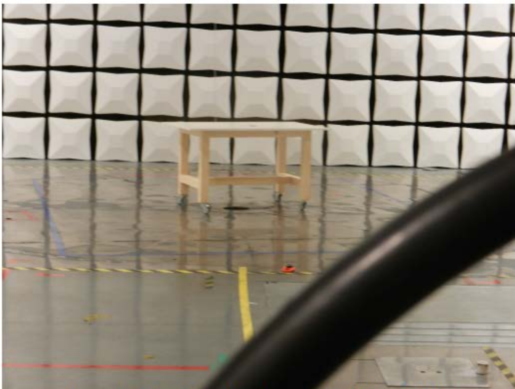
Figure 73 – Test Setup for frequencies 9 kHz – 30 MHz
