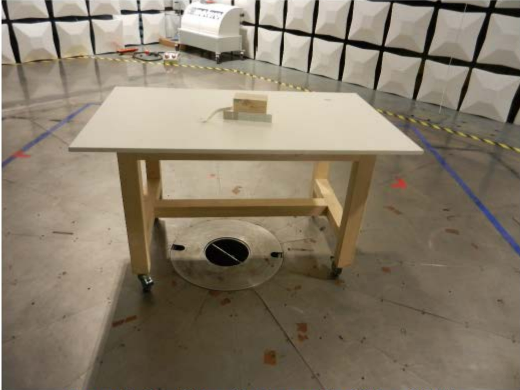
Figure 74 – Test Setup for frequencies 9 kHz – 30 MHz
