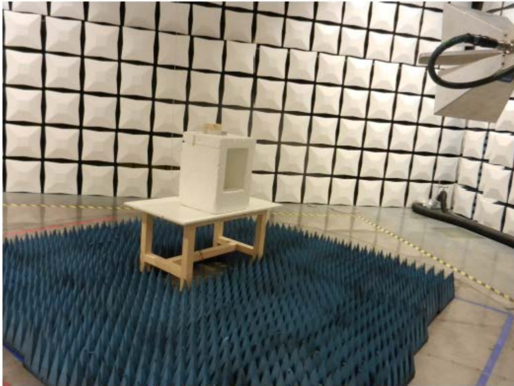
Figure 82 – Test Setup for frequencies >1 GHz
