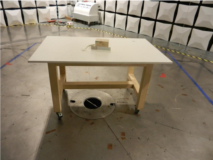
Figure 74 – Test Setup for frequencies 9 kHz – 30 MHz
