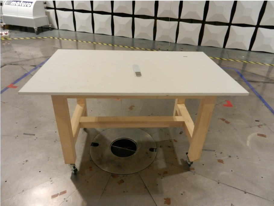
Figure 72 – Test Setup for frequencies 9 kHz – 30 MHz
