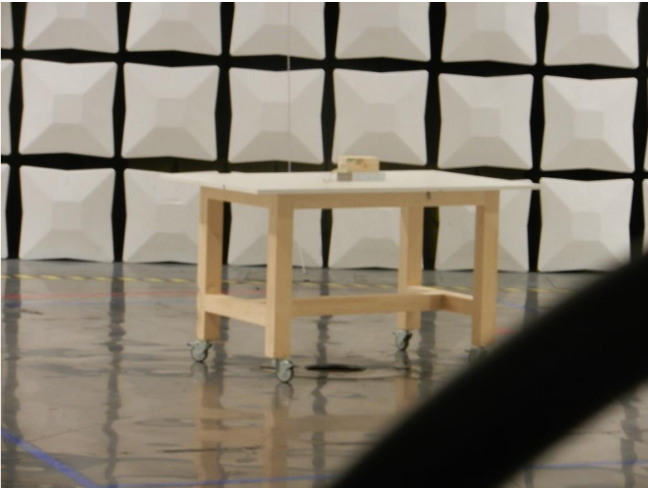
Figure 75 – Test Setup for frequencies 9 kHz – 30 MHz
