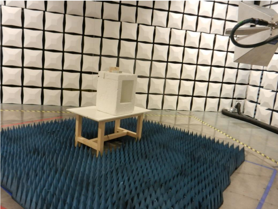
Figure 82 – Test Setup for frequencies >1 GHz
