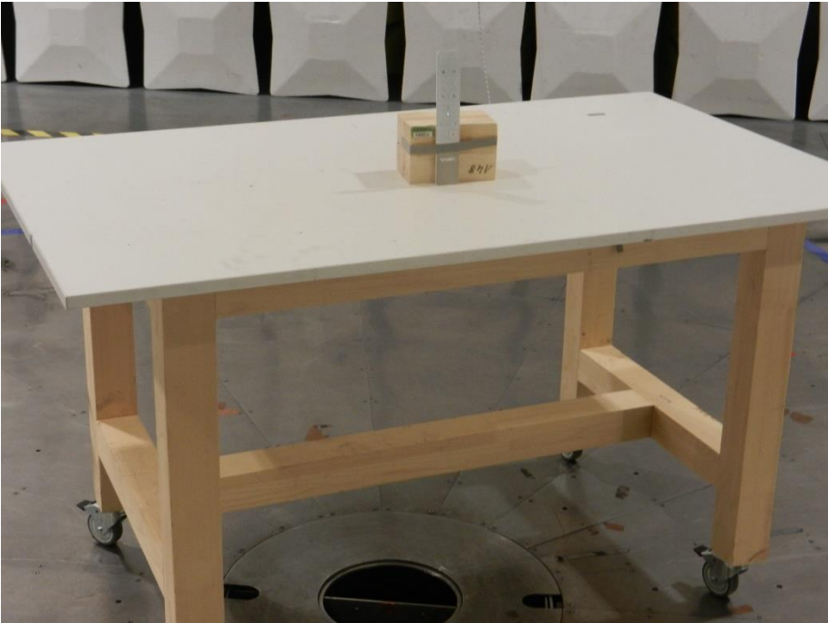
Figure 76 – Test Setup for frequencies 9 kHz – 30 MHz
