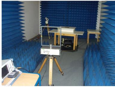
Test setup 30 MHz - 1000 MHz:
