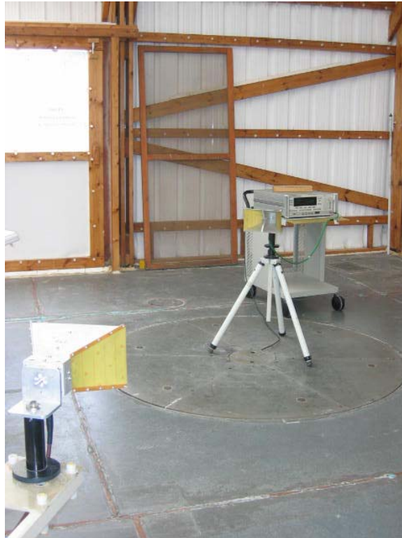
Photograph No.6 Setup for substitution ERP measurements of spurious at the OATS
