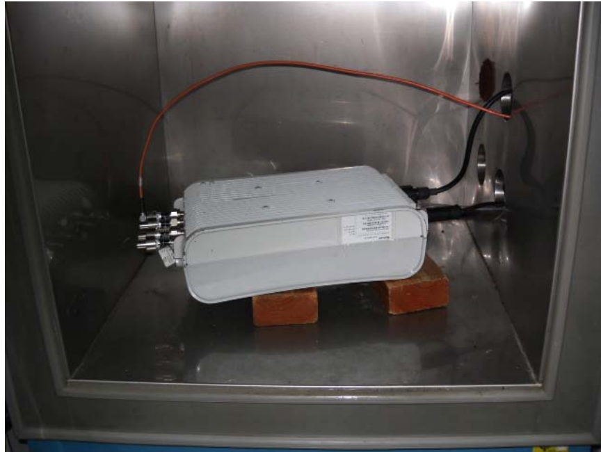
Photograph No.7 Frequency stability measurement setup
