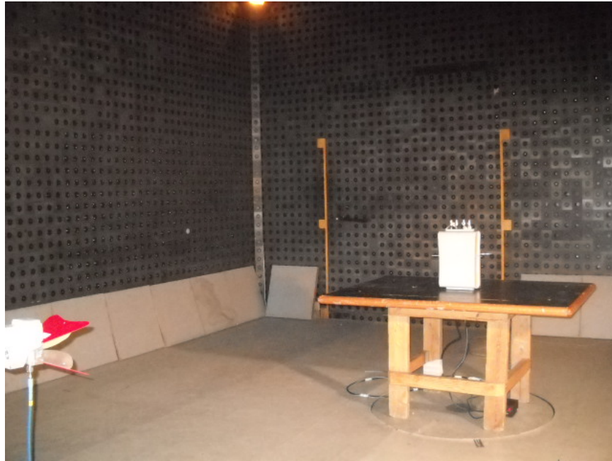
Photograph No.5 Radiated emissions measurement setup in the anechoic chamber in 1 - 18 GHz
