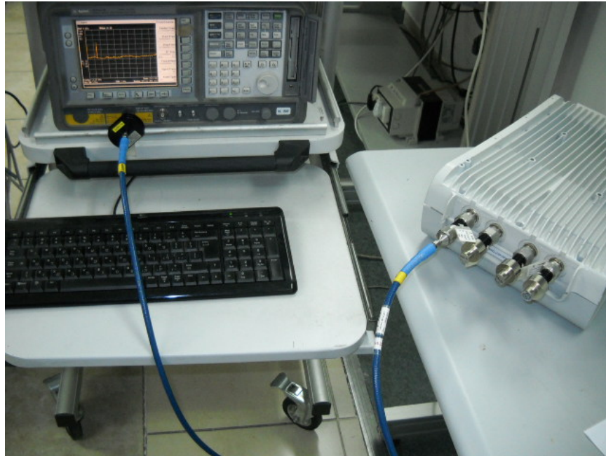
Photograph No.2 Conducted spurious emissions measurement setup
