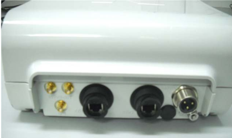
Photograph No.4 Pico base station side view
