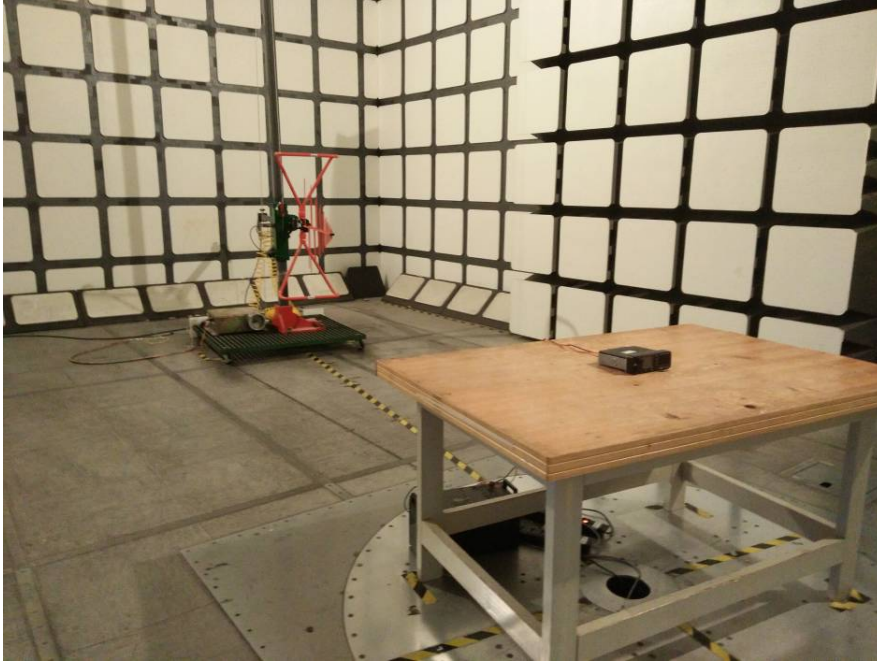
Radiated Emissions View (Below 1 GHz)
