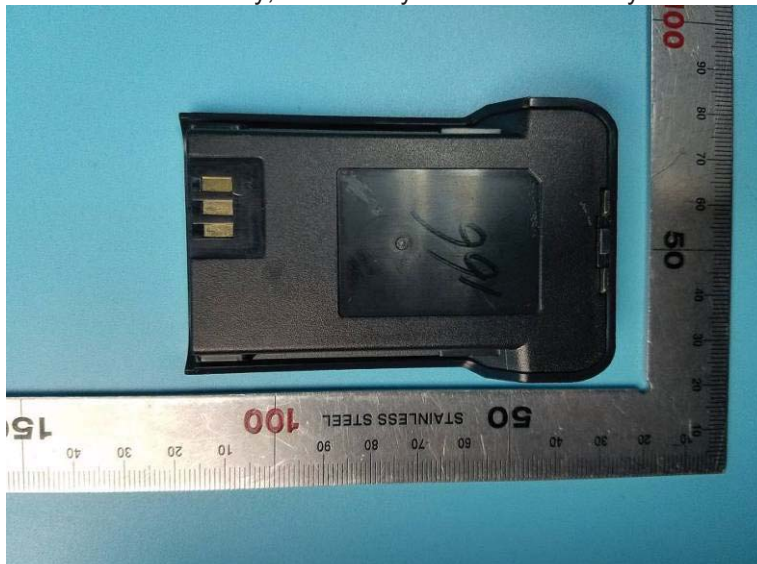
B1- Battery, Intrinsically Safe Li-ion Battery
