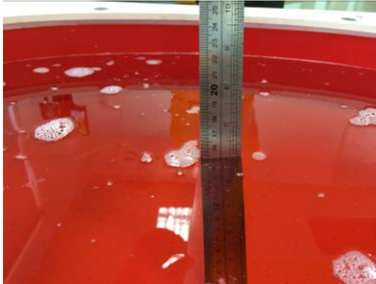
Photograph of the depth in the Head Phantom (150MHz)
