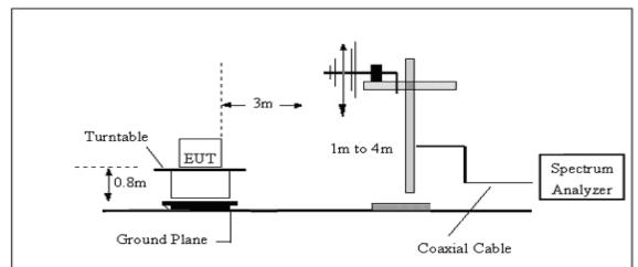
(C) Radiated Emission Test-Up Frequency Above 1GHz
