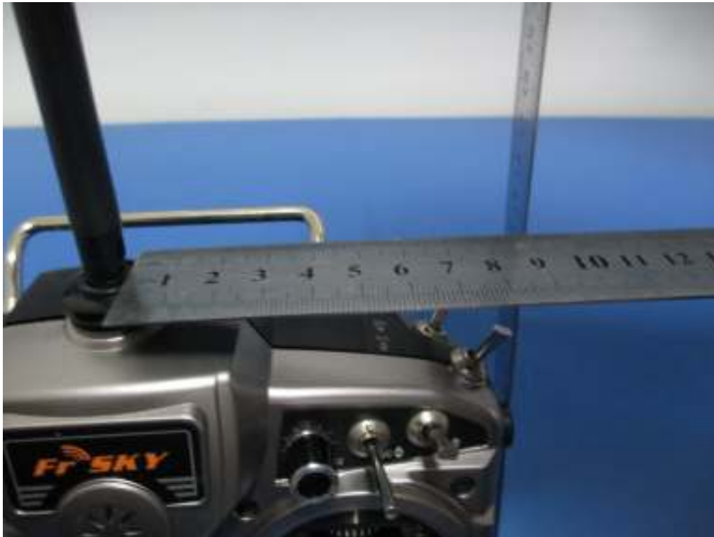
Antenna distance from right edge about 90mm
