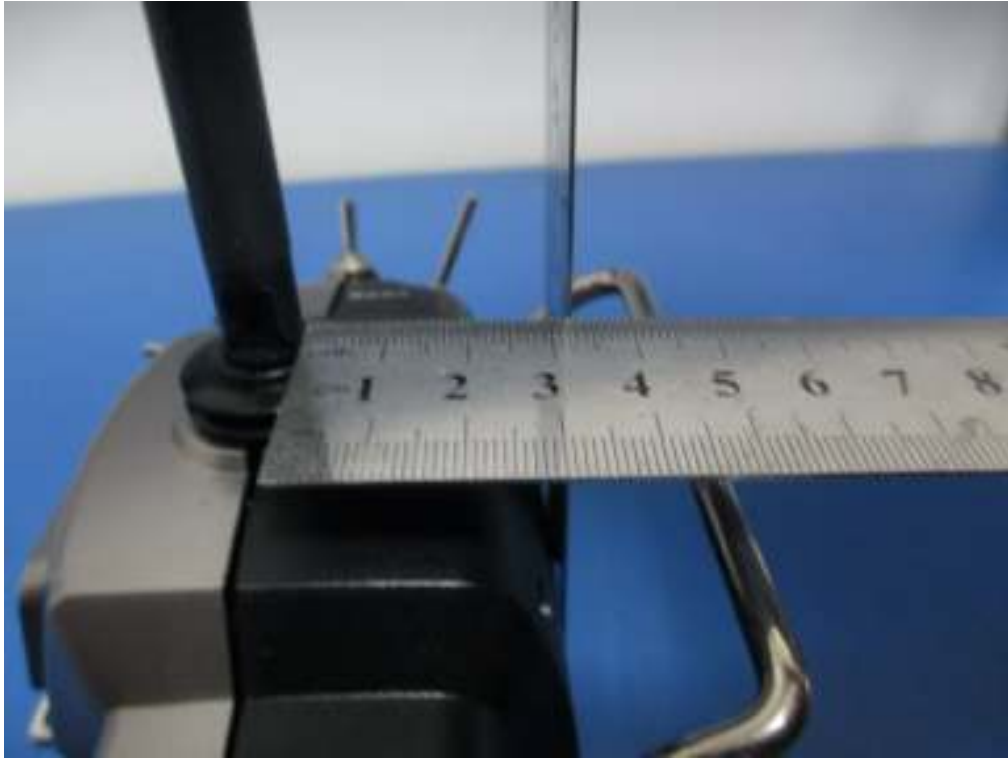
Antenna distance from Back surface about 33mm
