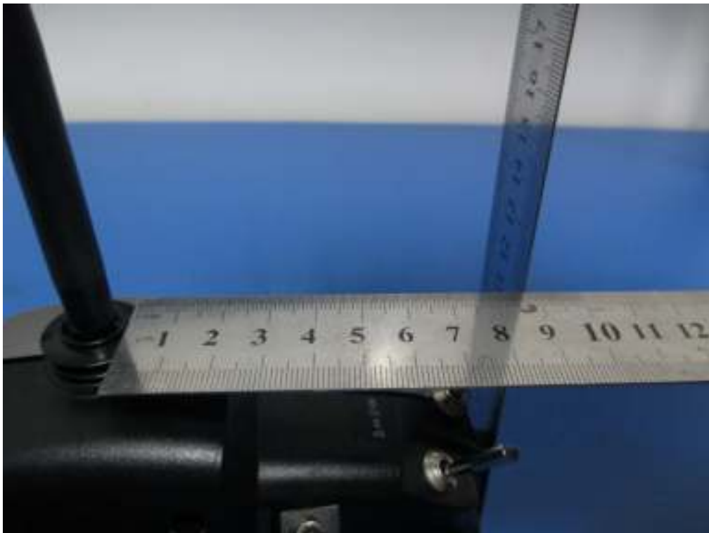
Antenna distance from left edge about 90mm
