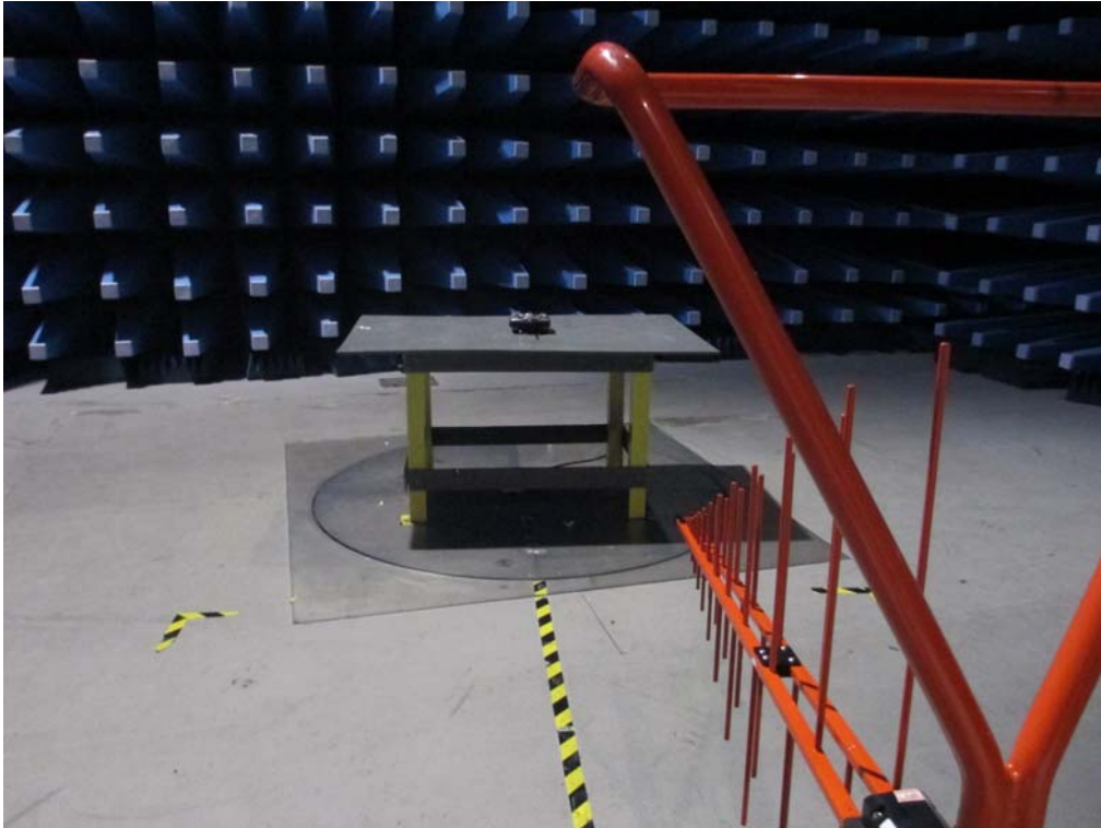
Radiated Emissions Test Setup Below 1GHz - Rear View
