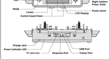
Notice: You can choose the Switch and define its positions in the Mixer menu. The DIY switch port is a free replacement switch position
