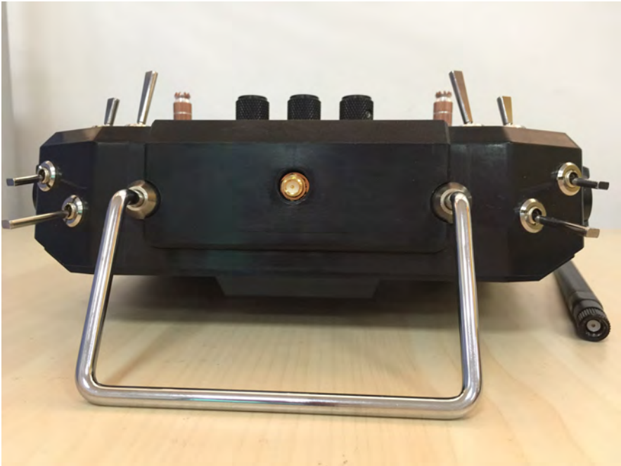
EUT – SRD Antenna Connector View
