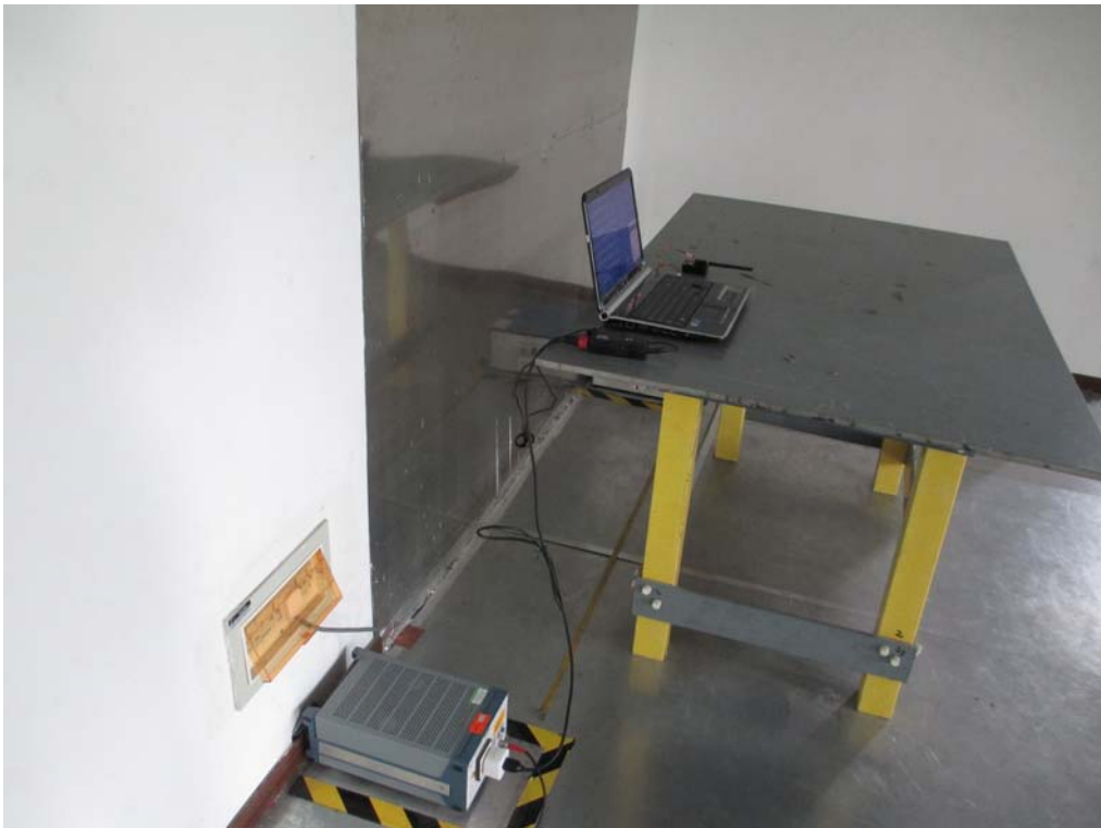
Conducted Emissions Test Setup Side View
