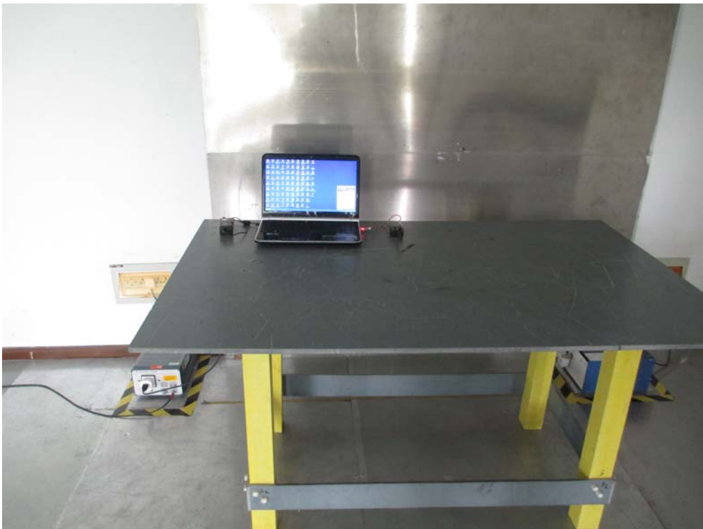
Conducted Emissions Test Setup Front View
