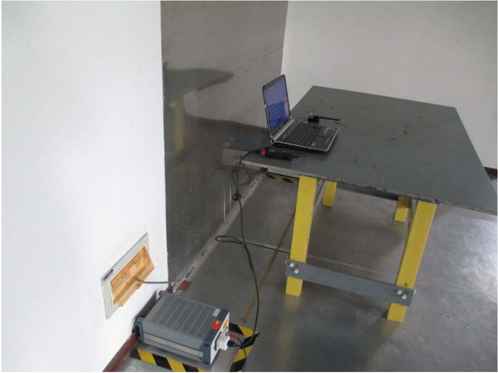
Conducted Emissions Test Setup Side View
