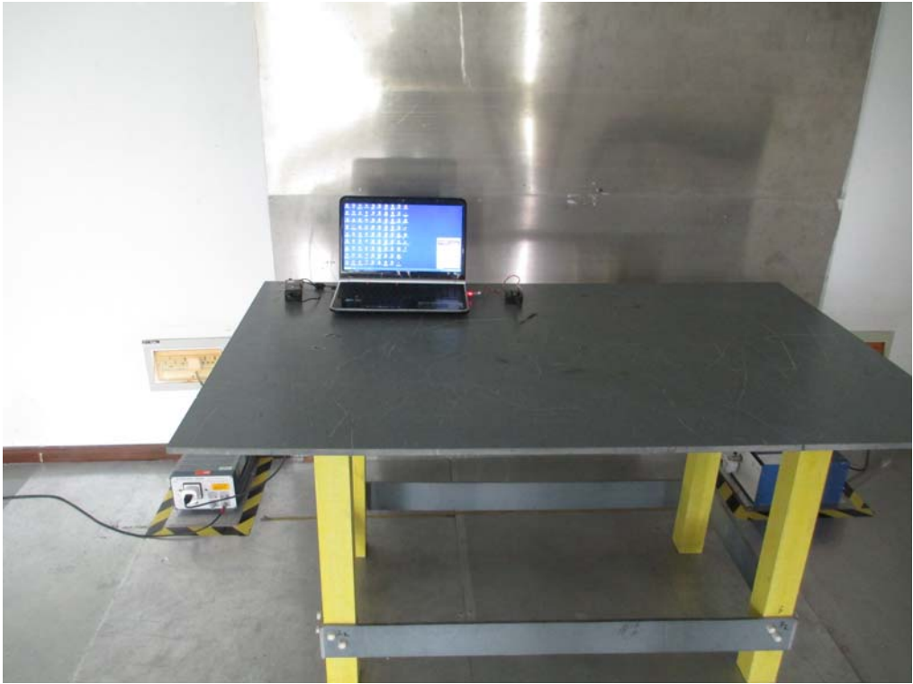
Conducted Emissions Test Setup Front View
