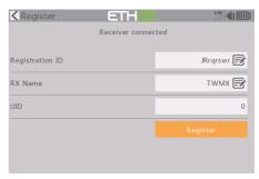
When the "RX Connected" page pops up, press the [REGISTER] to complete the Registration procedure and then power the receiver off.
