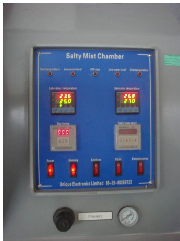
Figure 1.5 – View temperature of salt solution into reservoir
