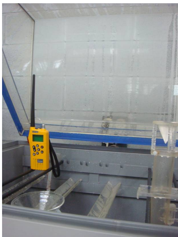
Figure 1.4 – EUT in the salt fog chamber
