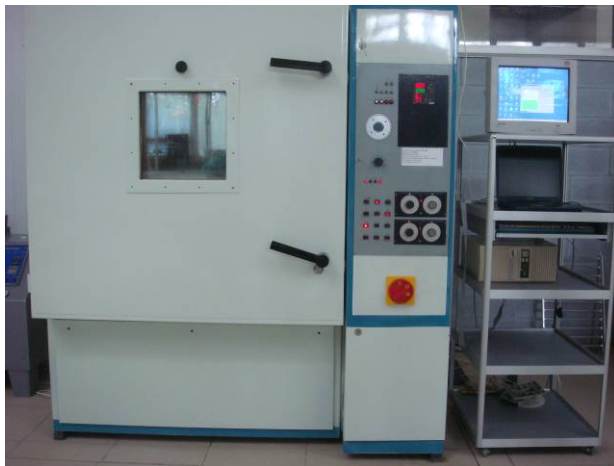
Figure 1.6 – EUT in climatic chamber
