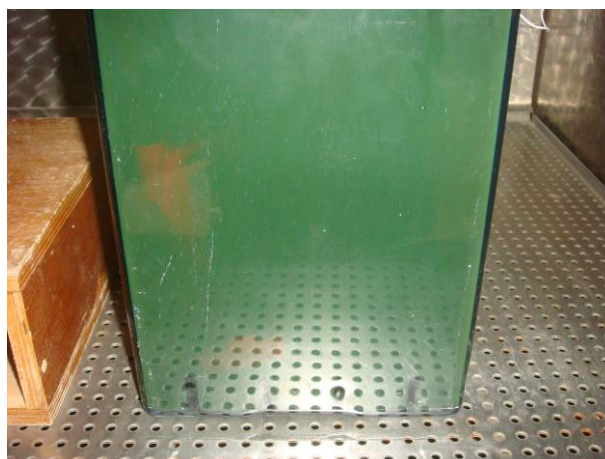
Figure 2.4 –EUT immersed in a tank with oil.
