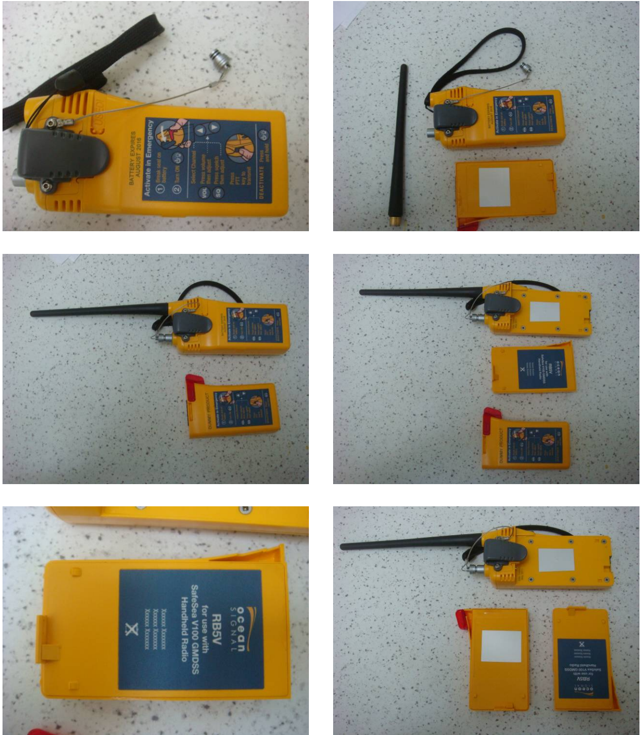
Figure 2.8 – Detail photo of parts of VHF Radio after the test
