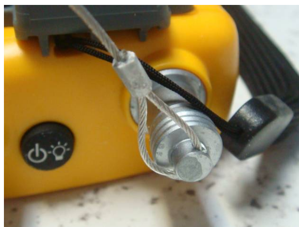
Figure 1.10 – Detail photo of parts of VHF Radio after the test. There are no corrosion, and other signs of deterioration
