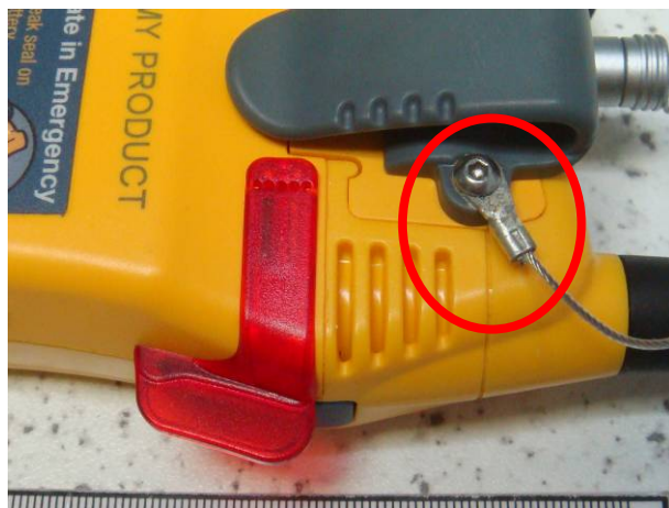
Figure 1.11 – Detail photo of parts of VHF Radio after the test There are no corrosion, and other signs of deterioration on all parts, except for the accessory socket dust cap cable clamp.
