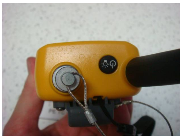
Figure 1.12 – Detail photo of parts of VHF Radio after the test There are no corrosion, and other signs of deterioration
