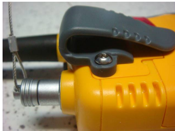
Figure 1.8 – Detail photo of parts of VHF Radio after the test. There are no corrosion, and other signs of deterioration
