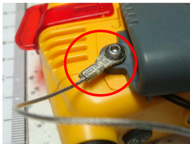
Figure 1.9 – Detail photo of parts of VHF Radio after the test. There are signs of deterioration of clamp
