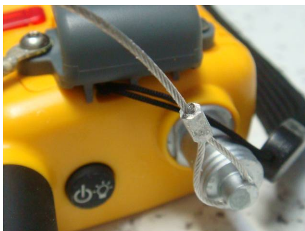
Figure 1.10 – Detail photo of parts of VHF Radio after the test. There are no corrosion, and other signs of deterioration
