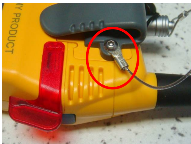
Figure 1.9 – Detail photo of parts of VHF Radio after the test. There are signs of deterioration of clamp
