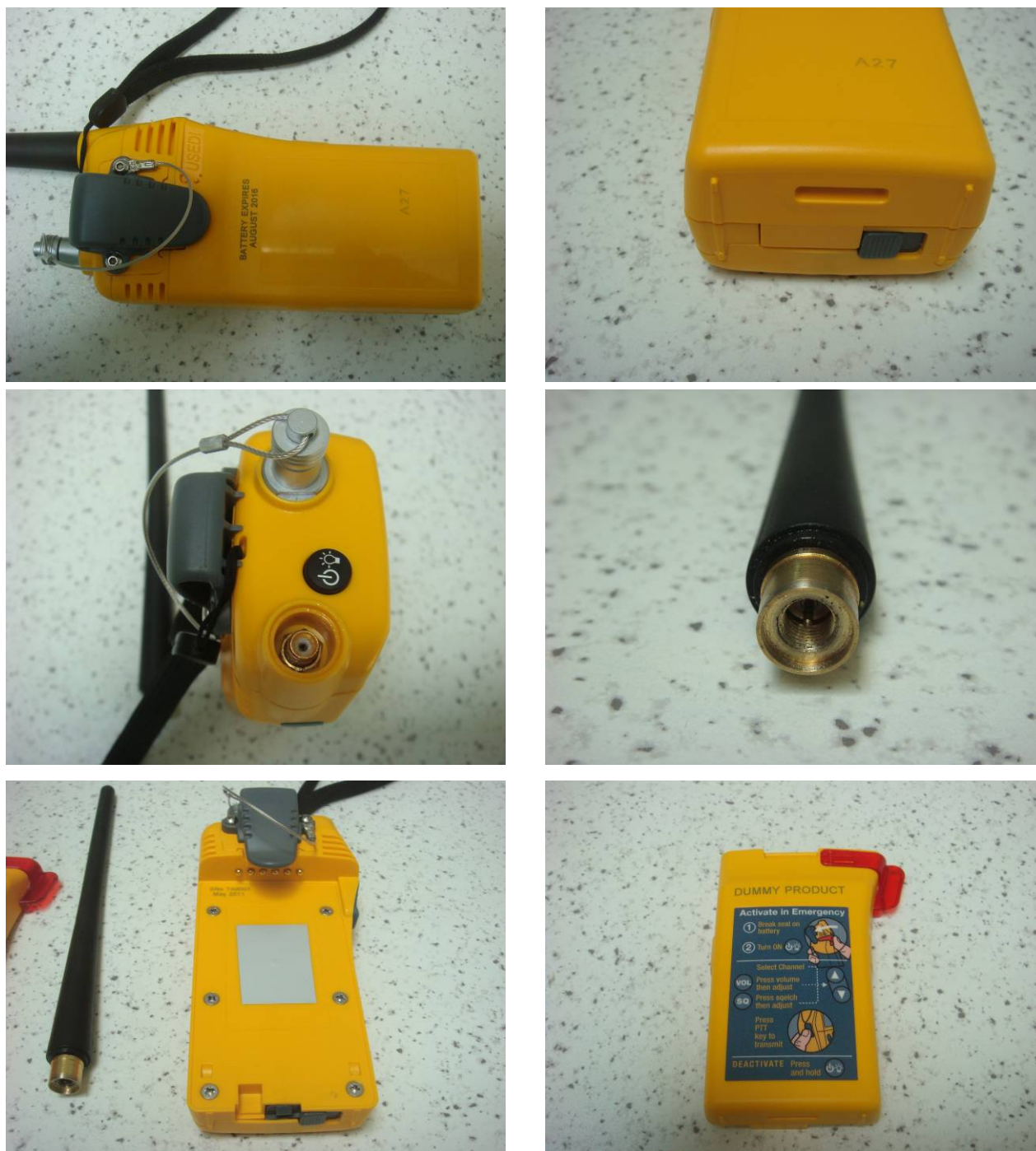
Figure 2.2 – Detail photo of parts of VHF Radio before the test
