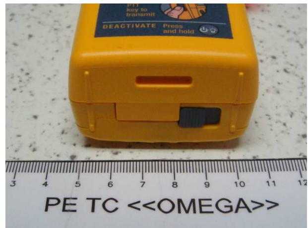
Figure 1.11 – Detail photo of parts of VHF Radio after the test There are no corrosion, and other signs of deterioration on all parts, except for the accessory socket dust cap cable clamp.
