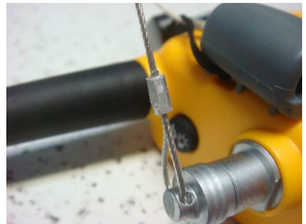
Figure 1.8 – Detail photo of parts of VHF Radio after the test. There are no corrosion, and other signs of deterioration
