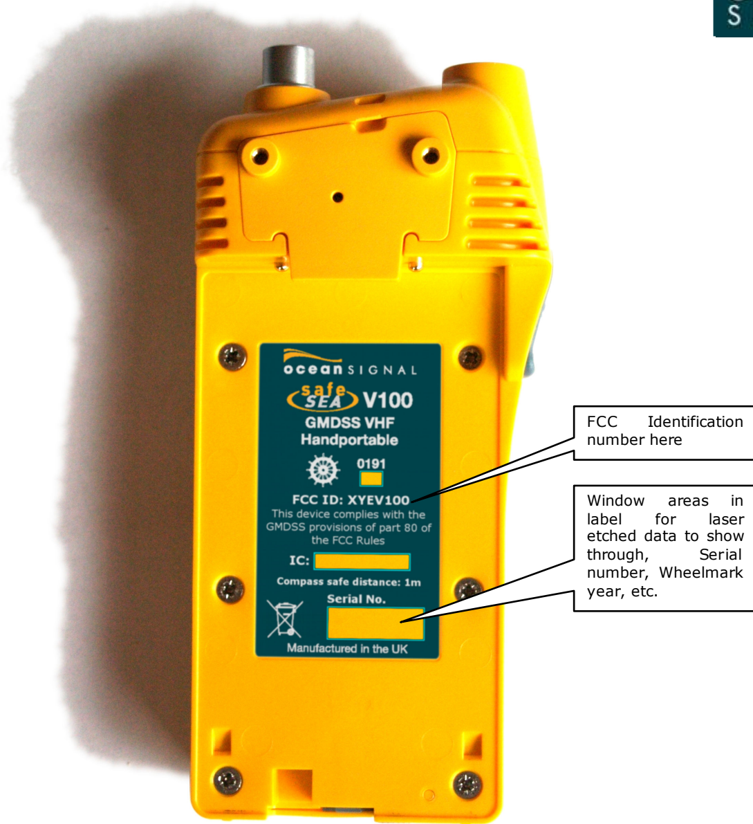
Figure 6: V100 Rear View with battery removed showing approvals label.
