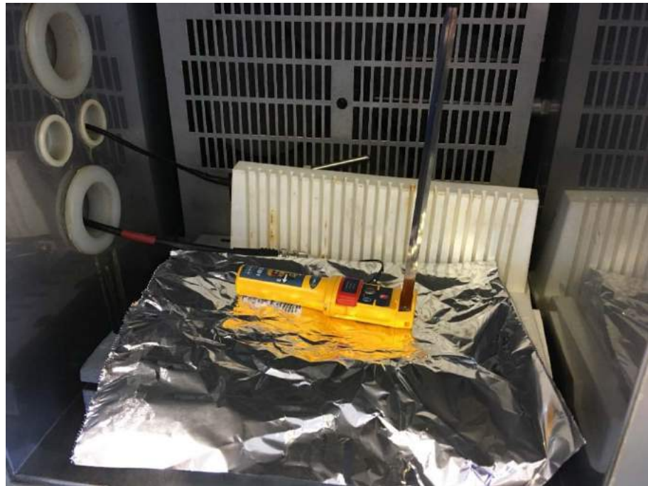
EUT – Battery Capacity Test
