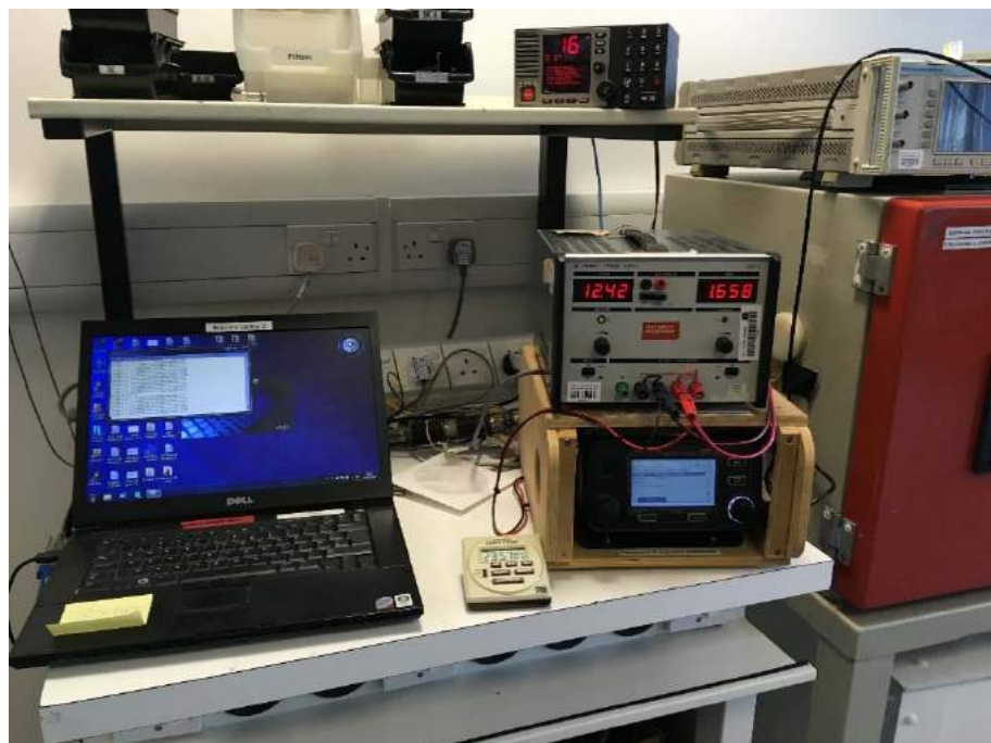
Battery Capacity Test Monitoring Equipment
