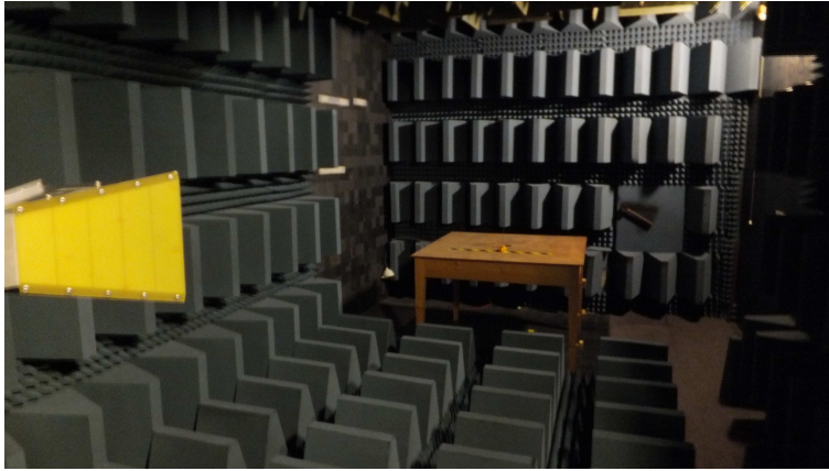
Figure 3: View of Anechoic chamber with microwave horn antenna. (Used for emissions above 1GHz)
