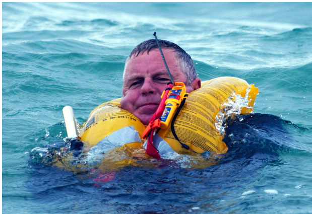
Figure 6 MOB1 showing antenna deployed and typical operational situation
