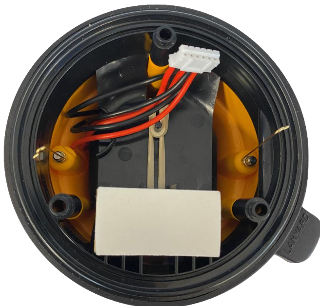
Figure 2: EPIRB3/EPIRB3 Pro – Top view, PCB removed showing battery carrier in-situ.
