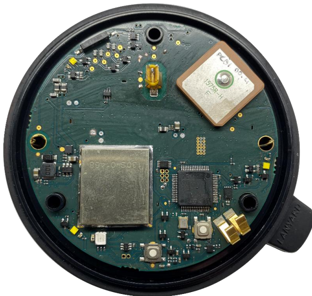
Figure 1: EPIRB3/EPIRB3 Pro – Top view showing PCB in-situ.
