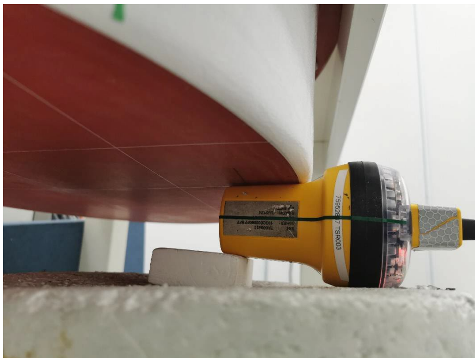
Figure 4. Right side of the DUT facing phantom, 0mm
