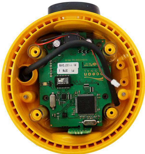
Figure 2: E101V EPIRB – Top view, EPIRB PCB removed, Showing VDR memory capsule PCB
