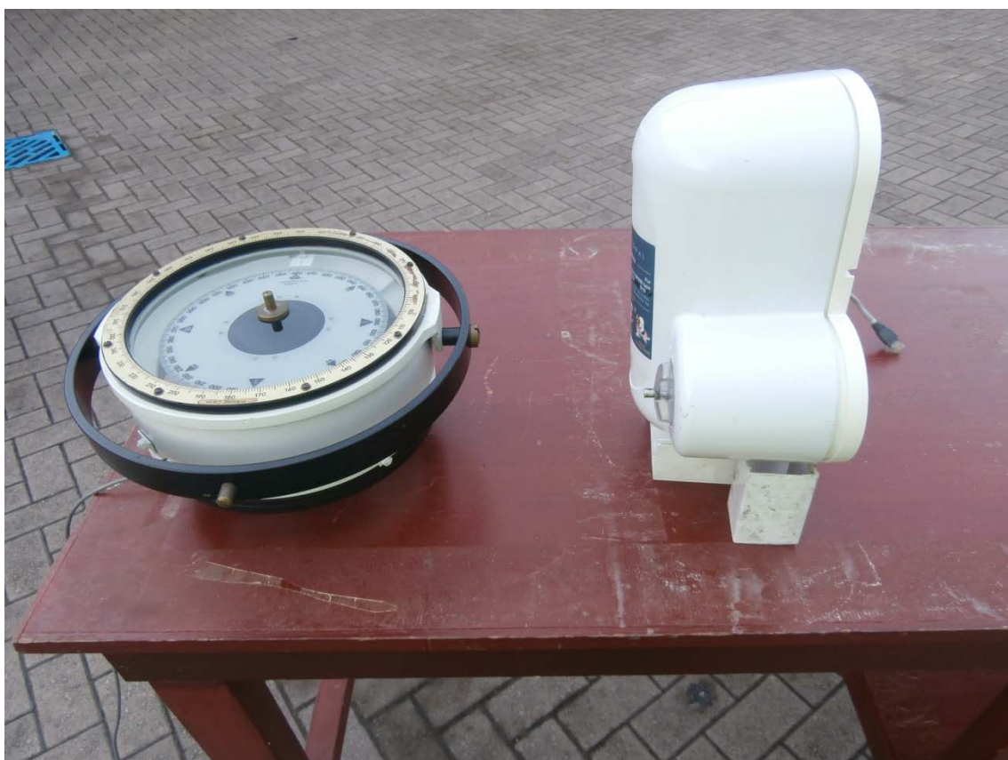
Compass Safe Distance Test (EUT in housing)
