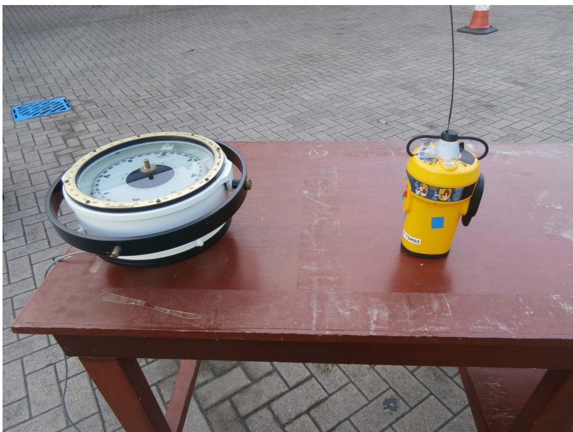
Compass Safe Distance Test (EUT standalone)
