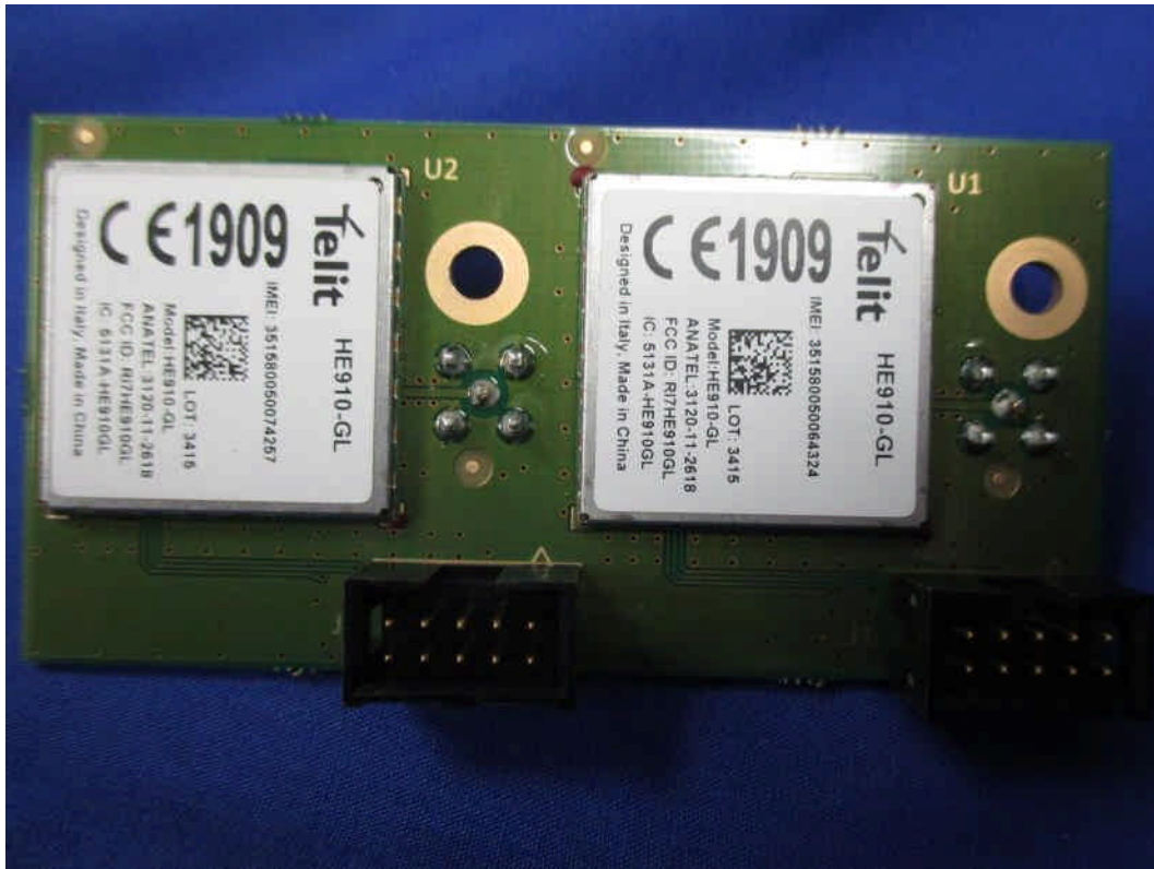
Close up 3G modems underside
