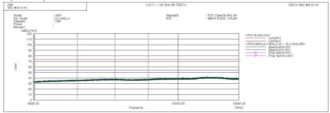
it was determined that X orientation was worst-case orientation; therefore, al final radiated testing was performed with the EUT in X orientation.
