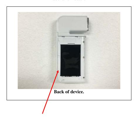
Label is placed inside of the battery compartment.
