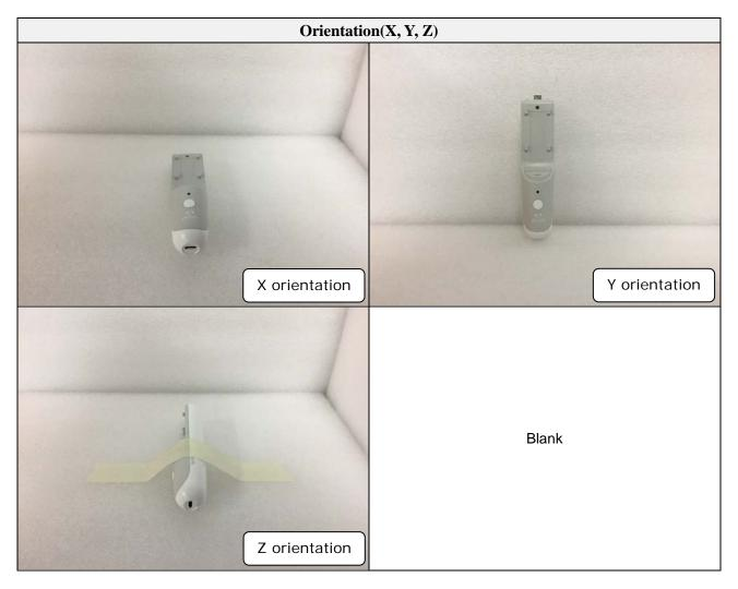
Note.: Radiated testing was performed with the EUT in worst-case Y orientation.
