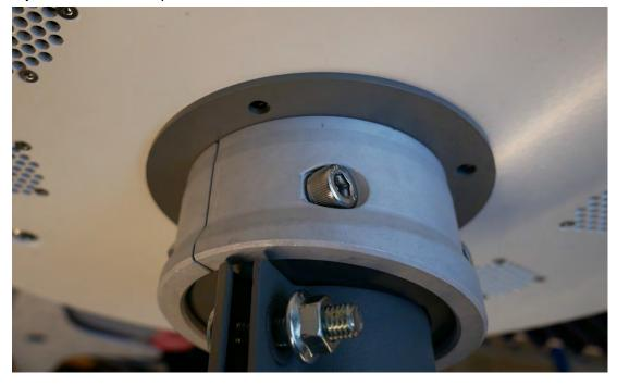
Figure 16: Antenna on Adjustable Mount Adapter
