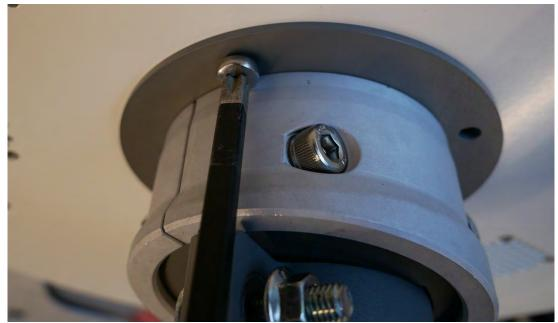
Figure 17: Attach Antenna to Adjustable Mount Adapter
