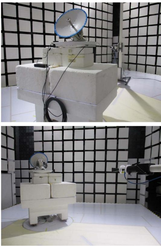
Radiated emissions measurements 18GHz to 26.5 GHz
