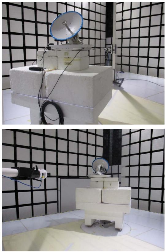
Radiated emissions measurements 26.5 GHz to 40 GHz
