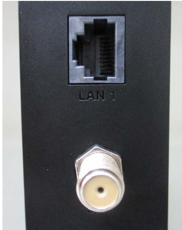
Customer Network Exchange I/O port
