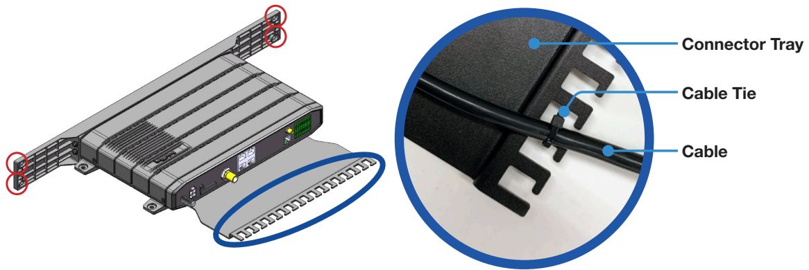
Figure 22: Mount BDU Assembly into 19" Rack
