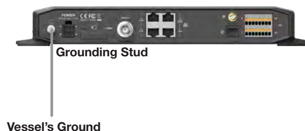
Figure 35: Grounding Stud Connection
