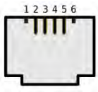
RJ14 & 6P4C (6-Positions 4-Contacts)
