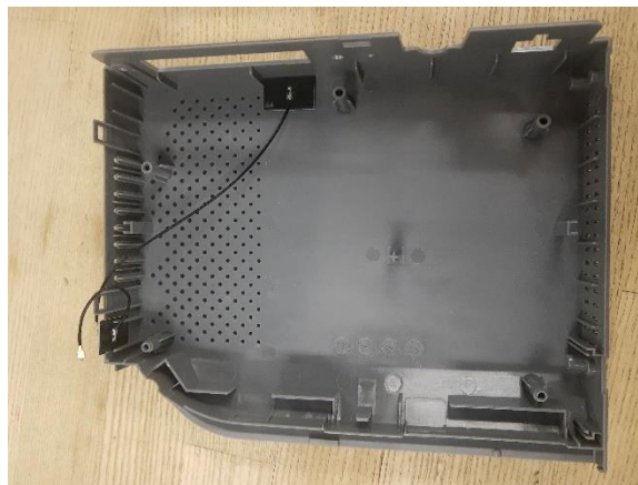
Photograph 10. CNX-WiFi, Internal 5 GHz Antenna Position
