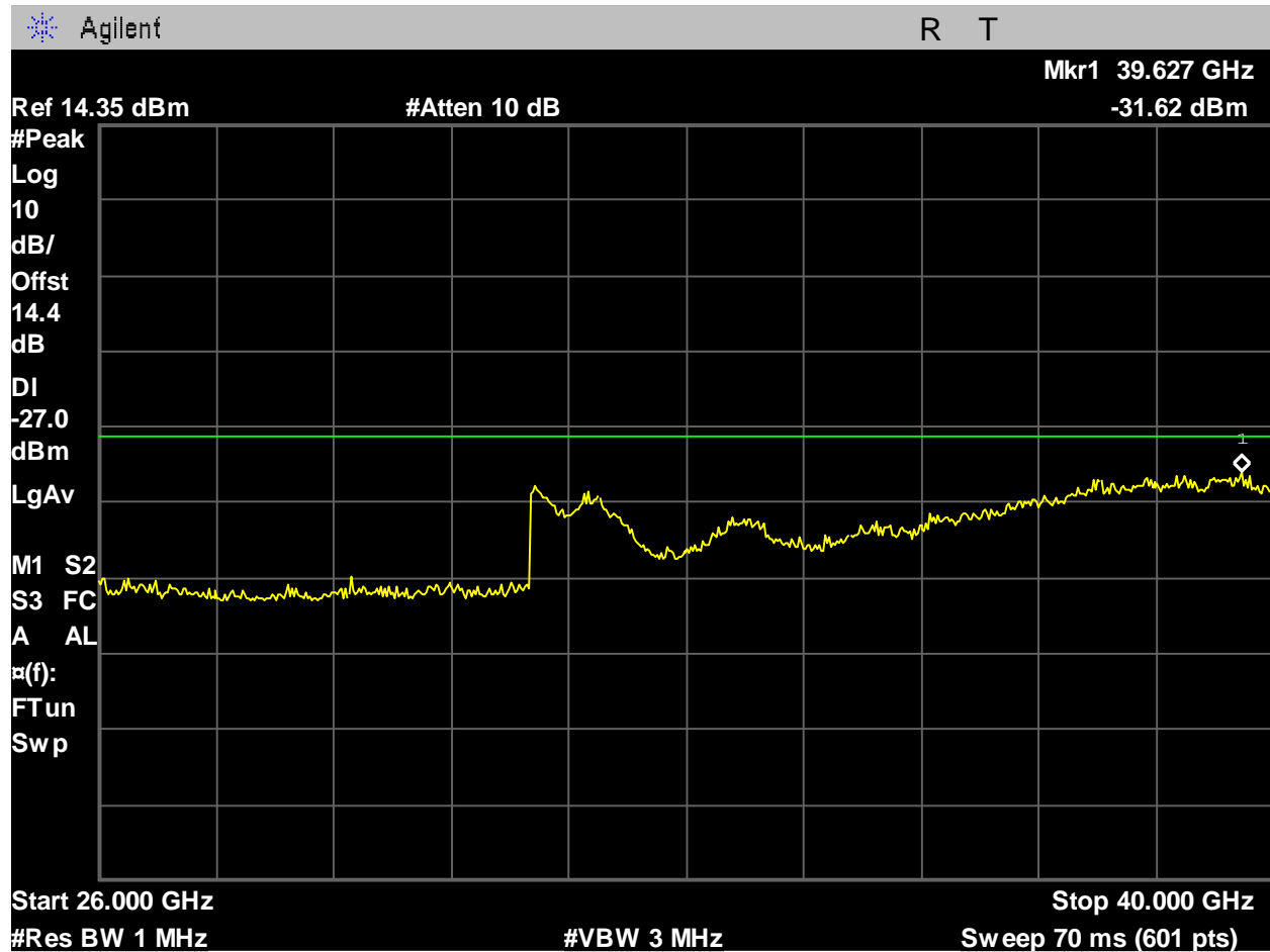
Figure 439: U-NII-3_5825MHz_High Ch_165_20MHz BW_n-mode_-27dBm_26-40GHz_Port 1.
