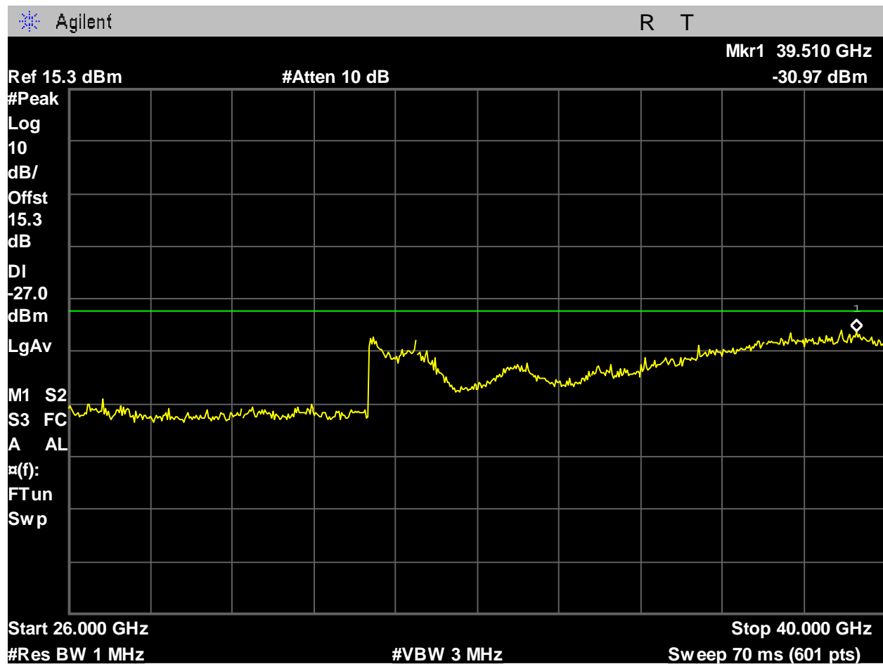
Figure 400: U-NII-3_5785MHz_Mid Ch_157_20MHz BW_n-mode_-27dBm_26-40GHz_Port 2.
