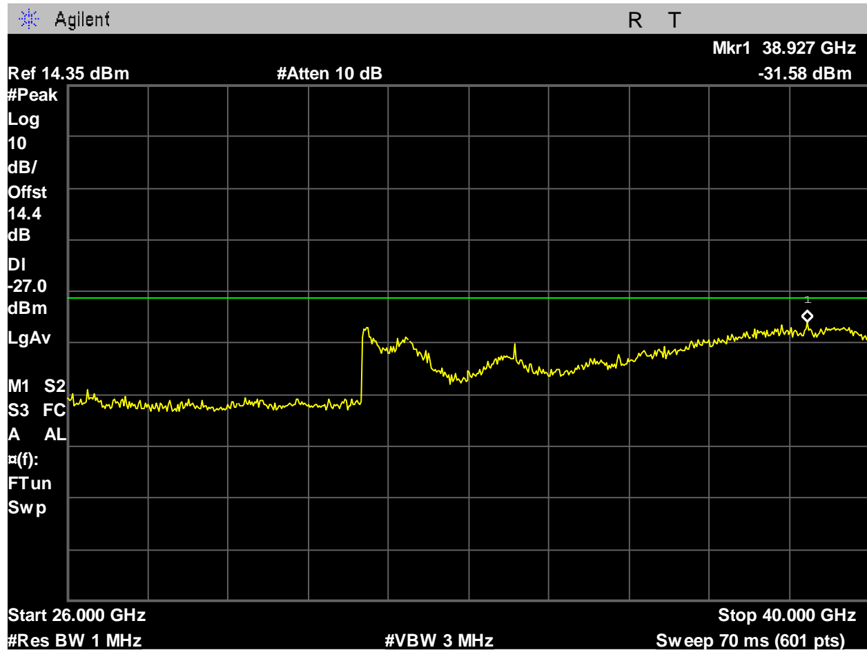
Figure 357: U-NII-3_5755MHz_Low Ch_151_40MHz BW_ac-mode_-27dBm_26-40GHz_Port 1.
