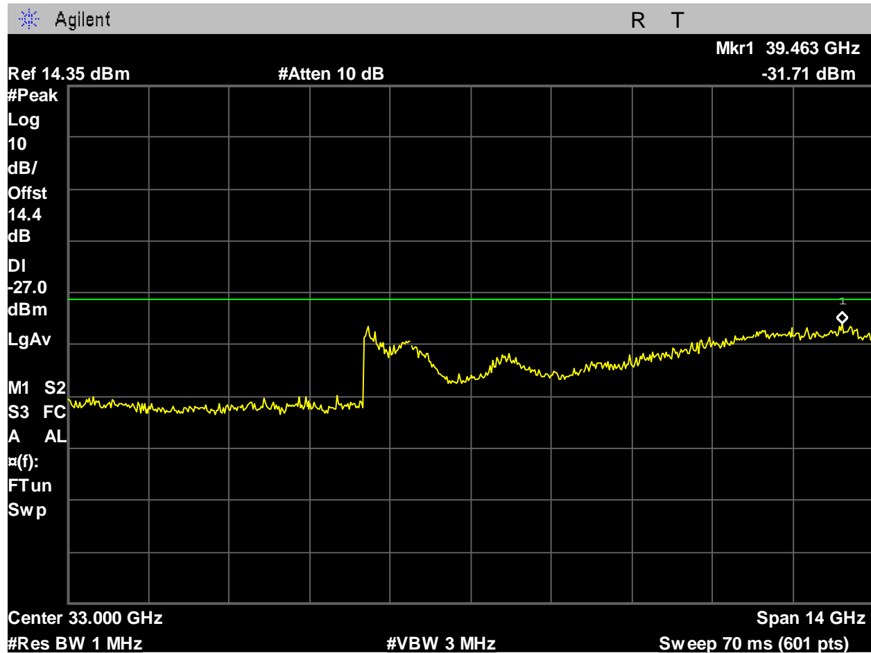
Figure 351: U-NII-3_5745MHz_Low Ch_149_20MHz BW_n-mode_-27dBm_26-40GHz_Port 1.
