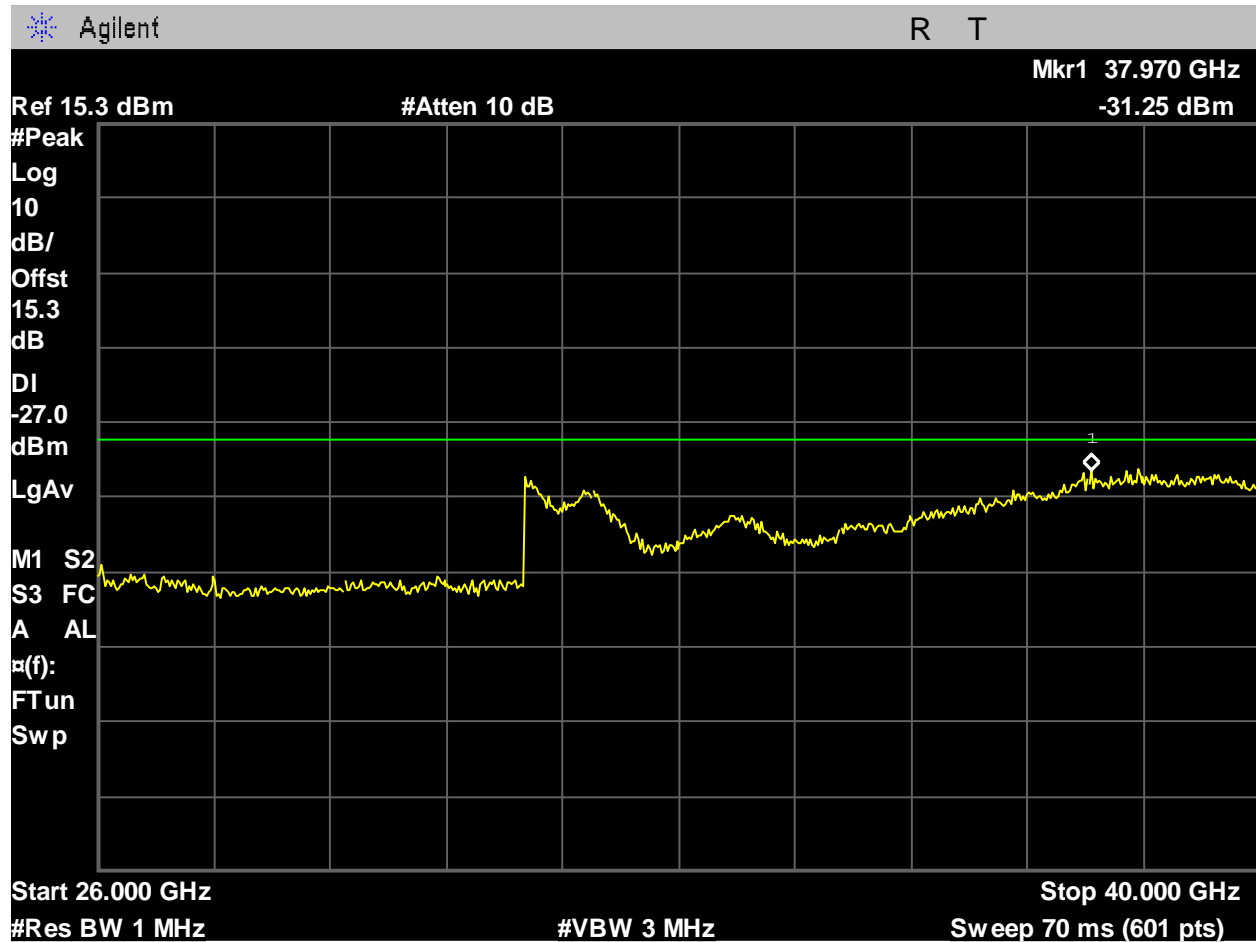
Figure 428: U-NII-3_5825MHz_High Ch_165_20MHz BW_ac-mode_-27dBm_26-40GHz_Port 2.
