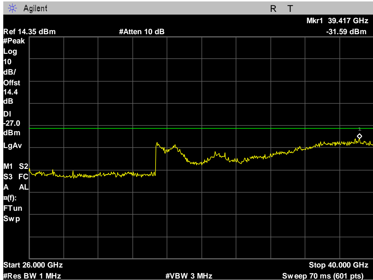
Figure 333: U-NII-3_5745MHz_Low Ch_149_20MHz BW_a-mode_-27dBm_26-40GHz_Port 1.
