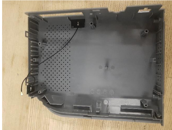
Photograph 10. CNX-WiFi, Internal 5 GHz Antenna Position
