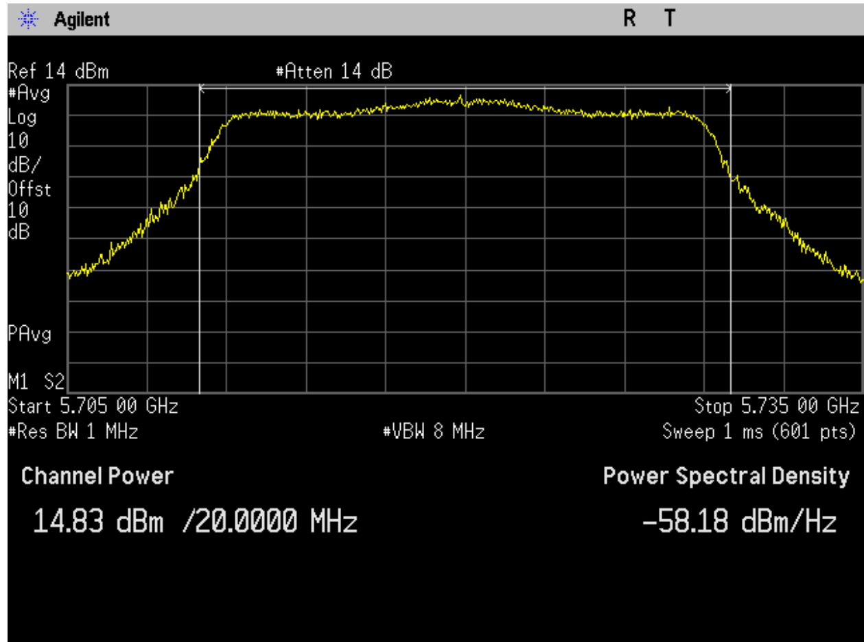
Figure 208: U-NII-2C_5720MHz_High Ch_144_20MHz BW_n-mode_Output Power_Port 2.
