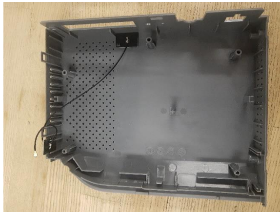
Photograph 10. CNX-WiFi, Internal 5 GHz Antenna Position
