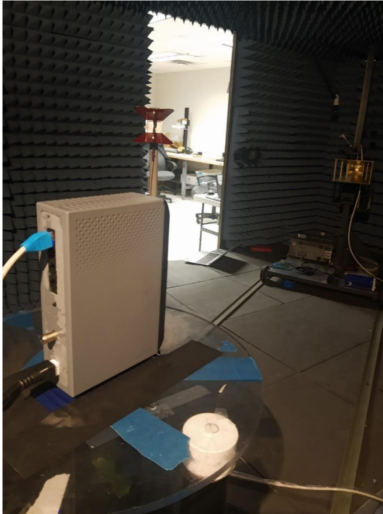
Photograph 13. DFS Test Setup
