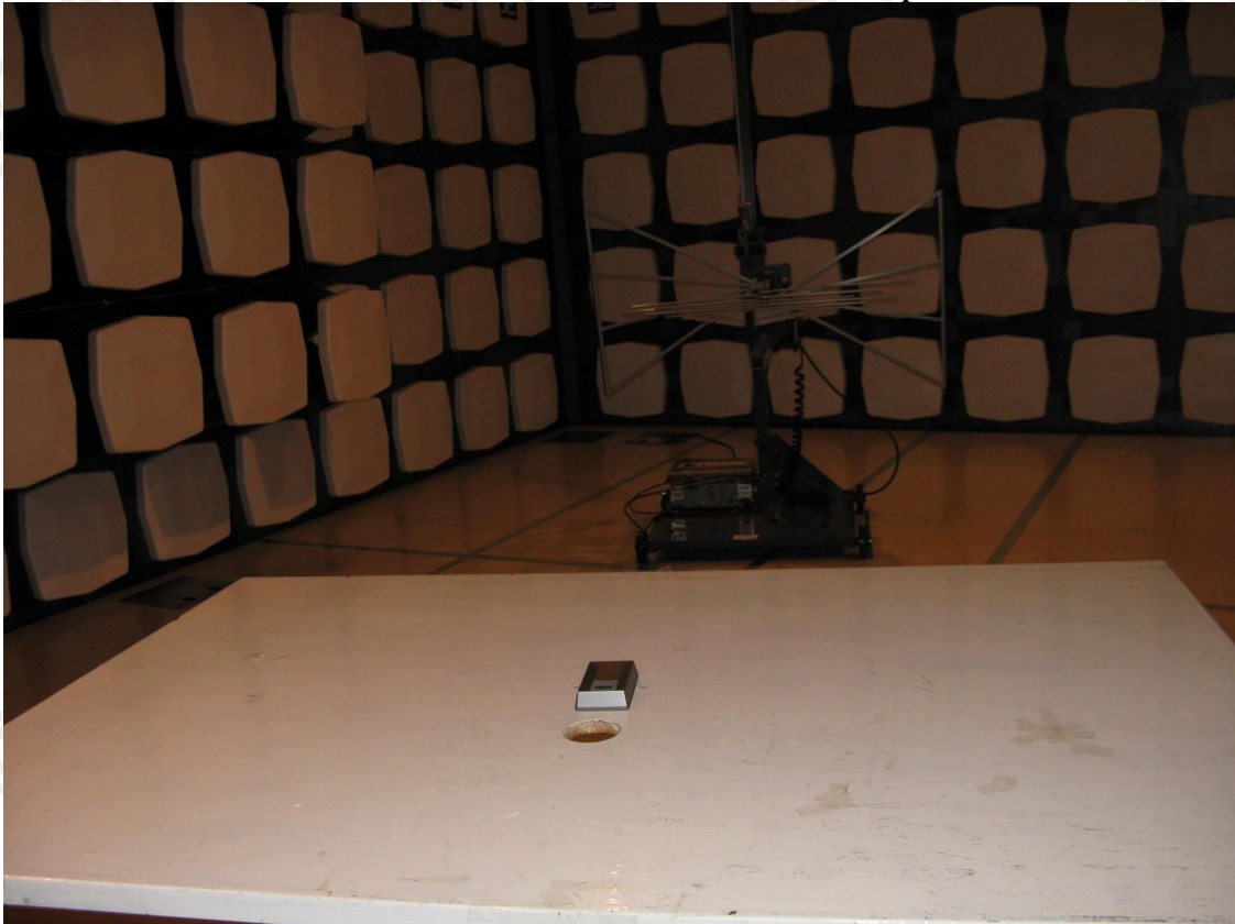
Measurement of Radiated Emission Test Set Up
