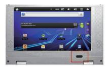
Turning On: To turn on the Netbook, press and hold the power button for 2 seconds until an image appears on the screen. Release the power button and let the software load on the Netbook. Please allow at least 45 seconds for the Netbook to fully start-up.
