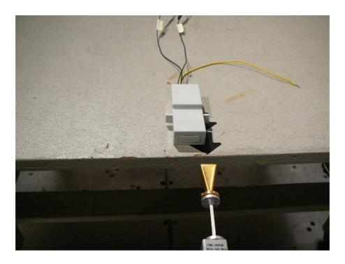
8.16 90 GHz to 120 GHz Radiated Emissions - Rear View
