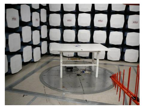
9.1 30 MHz – 1 GHz Radiated Emissions – Front View
