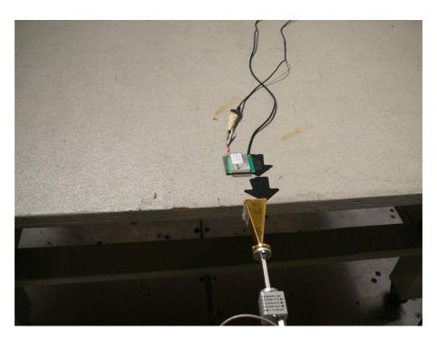
9.12 60 GHz to 90 GHz Radiated Emissions - Rear View
