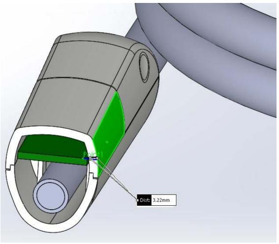
Note: The smallest distance from antenna to outer surface of the device is 3.22 mm.
